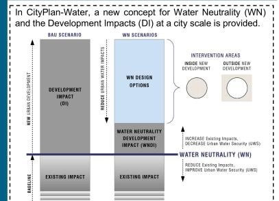
CityPlan-Water integrates Water Neutrality (WN) systemic design solutions with an Urban Water Security (UWS) evaluation toolkit, all being spatially represented in a GIS tool.
